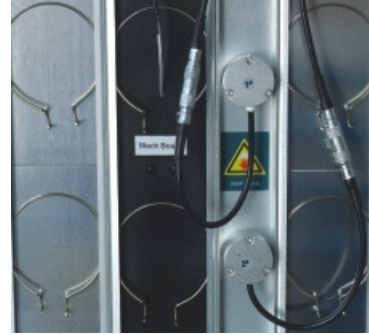
Four sensors monitor UV irradiance
