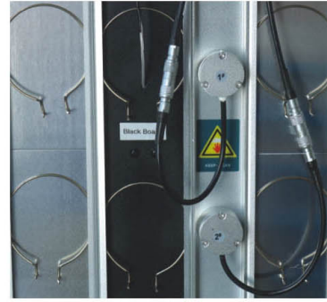
Four sensors monitor UV irradiance
